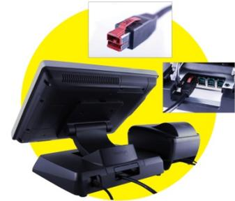
[Terminal and printer power brick is inside the base](#)
