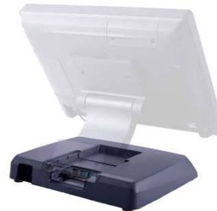
Posiflex XT Series of touchscreen terminals offers a base where its own power adapter can be integrated with an optional PoweredUSB and additional functionality on the Posiflex XT3215, XT3815, XT4015 and XT5315 terminals
