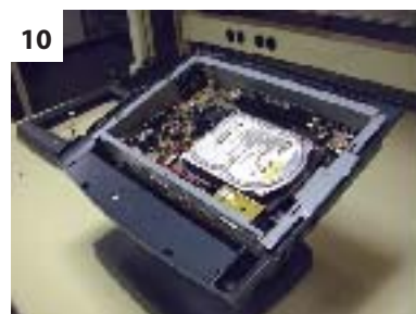
7 Remove "ONE" screw. Slide the metal plate down hard and lift plate to access hard drive and mainboard.
