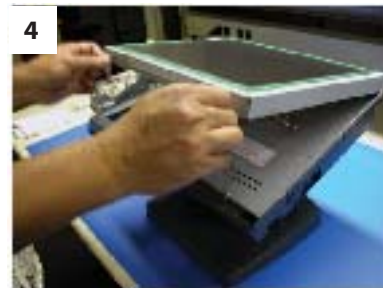
4 Lift up the LCD panel chassis
