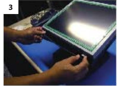
3 Pressing down on the two spring clips, lift both sides of the top LCD chassis to open
