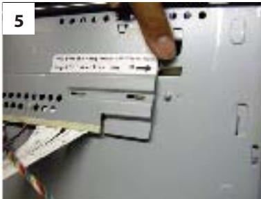
5 To remove the metal cover plate from the main chassis, press down on the spring button and slide cover to right to remove the riser card cover. Pull the riser card cover out, disconnect riser card and remove LCD chassis.
