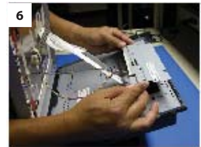
5 To remove the metal cover plate from the main chassis, press down on the spring button and slide cover to right to remove the riser card cover. Pull the riser card cover out, disconnect riser card and remove LCD chassis.
