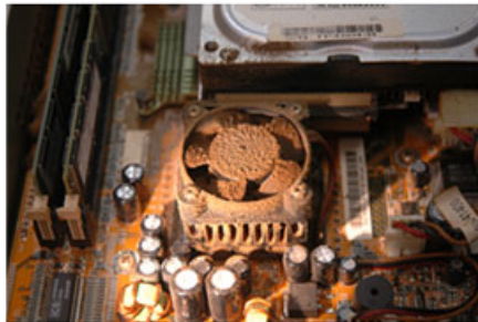
Interiors of typical fan-cooled systems with grease and dust build up on fans and heat sinks
